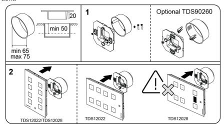
RECOMMANDED wall boxes: TDS90000 and TDS90000PB. The TDS90000 is used in brick walls, while the TDS90000PB is used in plaster board or wood panel walls.
