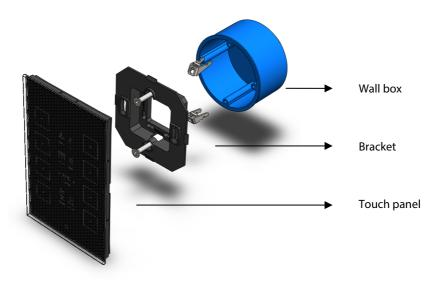
The design of the AURUS-OLED enables you to place the touch panel both vertical as horizontal. The choice is up to you or your customer. However, the AURUS-6 TEMP must be installed only vertically.
