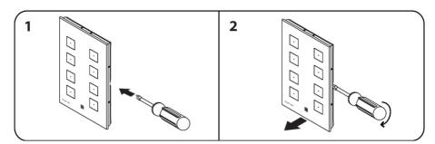
To remove the AURUS panel out of the wall bracket, place a flat screw driver into the holes at the sides of the AURUS panel. The wall bracket is provided with two clips which protect the wall during this action! Do not remove the AURUS-panels by pulling the glass front panel, or warranty will void.
