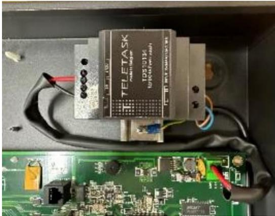
The intention is that we arrive at the result as shown in the picture on the left. The TDS10134 power supply is placed at the top right of the MICROS+ cabinet on a DIN rail instead of the 'old' power supply under the sealing cap (photo above).
