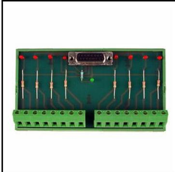
This module is 8 channels open collector output module.
