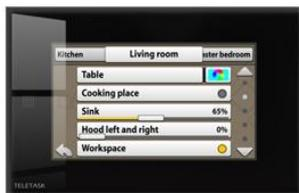
The TELETASK AURUS-TFT features a 4.3" colour wide screen touch panel with LED backlighting. Connection to AUTOBUS makes it a full featured central control panel, including IP camera view due to the Ethernet connection. In combination with the design phone (TDS20101), this touch screen also becomes an indoor unit of your analog- or IP- door video phone system.
